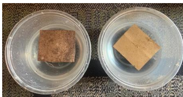
Figure 2. Koka-Paper (left) and cardboard (right) soaked in water
