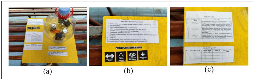
Figure 1. CADITEKS Design Components: (a) CADITEKS components, (b) how to use & safety procedures, (c) PPM indicators & observation results table
